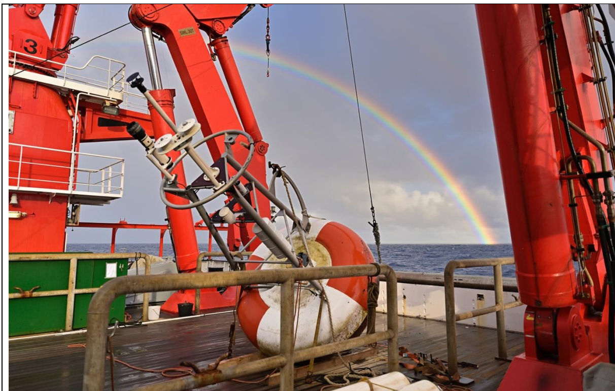
Figure 1: Head buoy of the PIRATA array on deck of RV SONNE. (Picture: Solvin Zankl)
