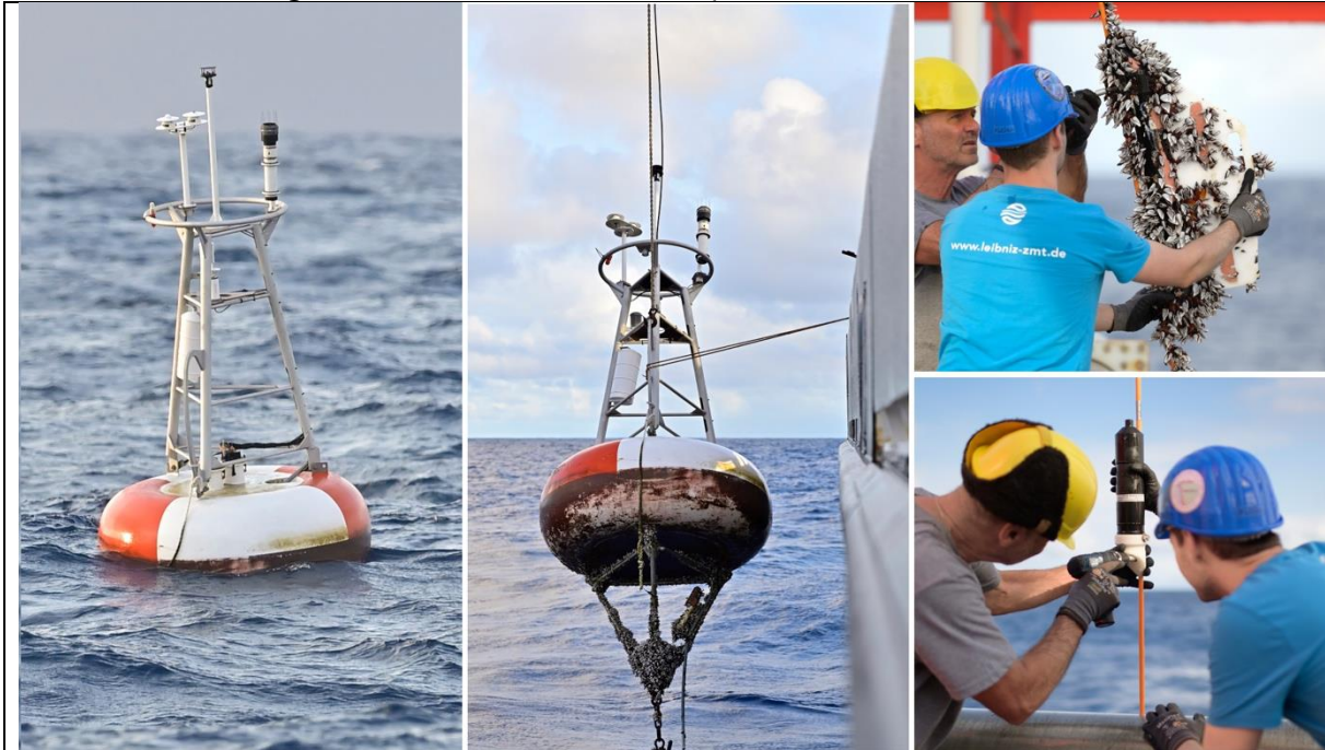
Figure 2: PIRATA head buoy drifting in the Atlantic Ocean and on a hook of RV SONNE as well as the recovery of scientific sensors from the cable below the head buoy. (Picture: Solvin Zankl)
