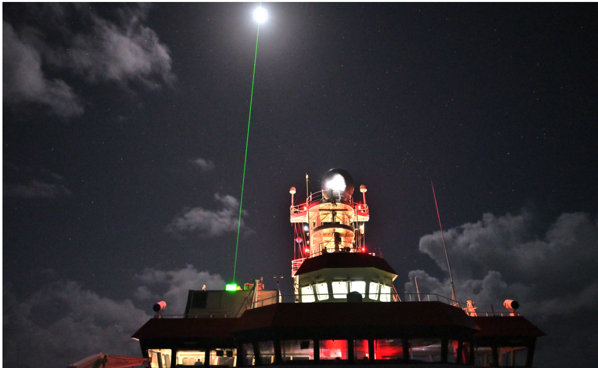
Figure 1 Night-time view of the 532nm laser beam from the PollyXT Lidar installed on RV Sonne during cruise SO284. The Lidar measures profiles of atmospheric humidity and aerosols.
