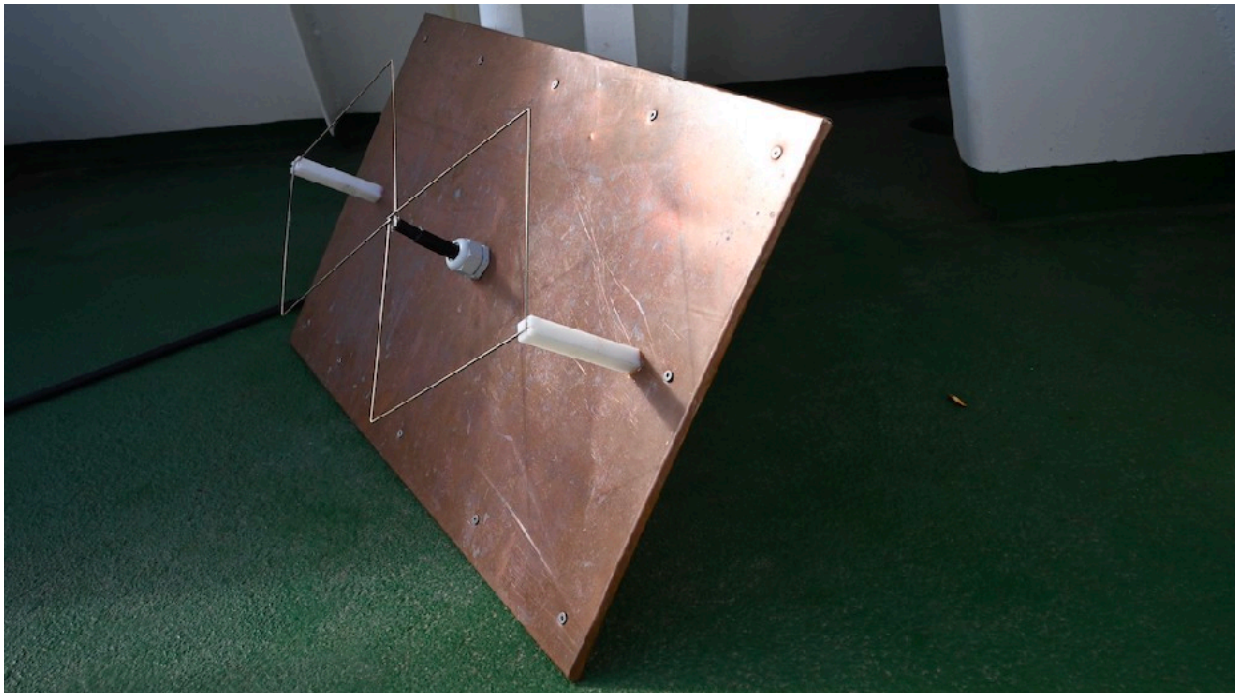
Fig. 2: Bi-Quad antenna built on board to amplify the measured radiosonde signal (© Julia Windmiller)
