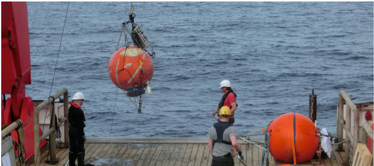
An ADCP with buoyancy body and other sensors are recovered and returned to the deck (© Universität Hamburg/Niko Lahajnar).
