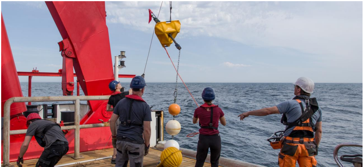
Teamwork: The head buoy of a drifter system is deployed (© University of Hamburg/Knut Heinatz).
