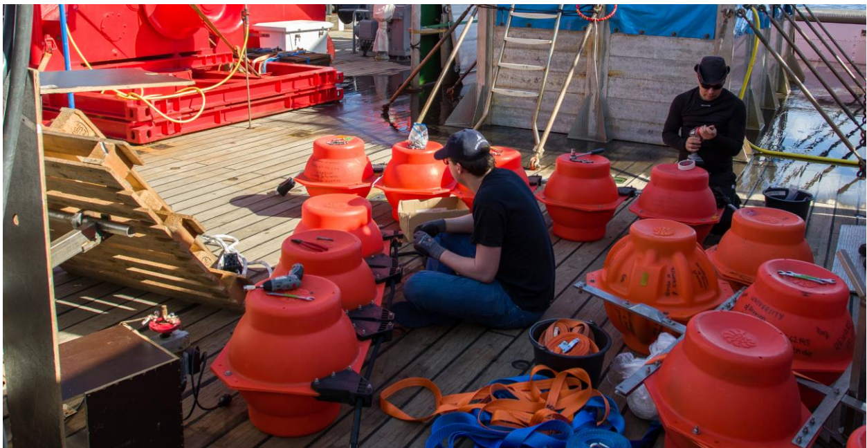
Flotation modules are prepared and assembled for the upcoming TRR181 program moorings (© Universität Hamburg/Knut Heinatz).
