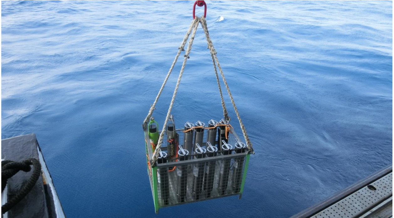
A cage full of acoustic releases goes on a test run in the depths of the Atlantic Ocean (© Universität Hamburg/Niko Lahajnar).
