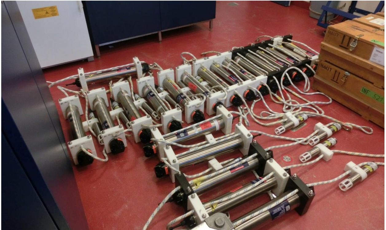
An impressive number of prepared current meters and temperature sensors for the TRR moorings in the South Atlantic (© Universität Hamburg/Niko Lahajnar)
