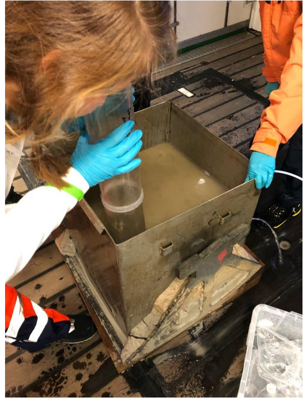
Figure 3. The sediment team subsampling cores from the box core. © I. Schulz/GEOMAR
