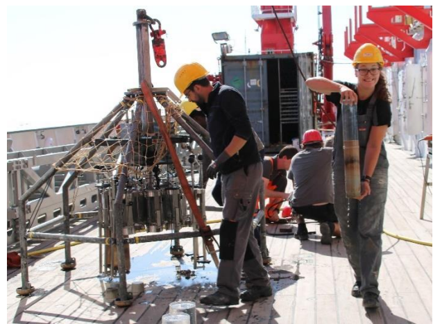
Figure 2: In addition to other sampling devices, the multicorer is always present on the working deck. By using it, the top 50 cm of the sea floor are sampled very precisely. (© Julia Krahl).
