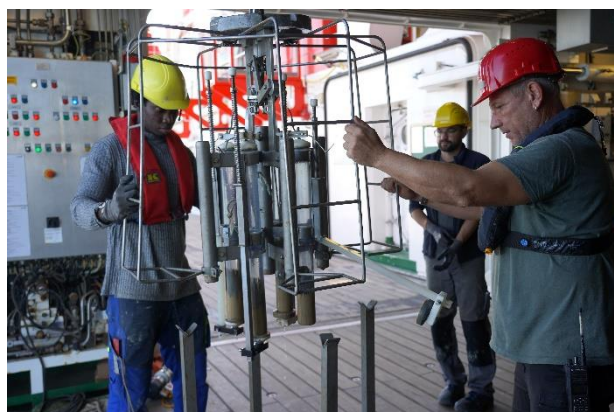
Figure 4: The minicorer, a very simple instrument for taking precise seabed samples with bottom water, is received on the ship (© Tabea König).
