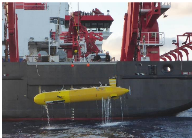
Figure 1: The MARUM AUV Seal 5000 is hoisted on deck with the A-frame on R/V SONNE after its 13-hour dive in 2000 m water depth (© Till von Wahl).
