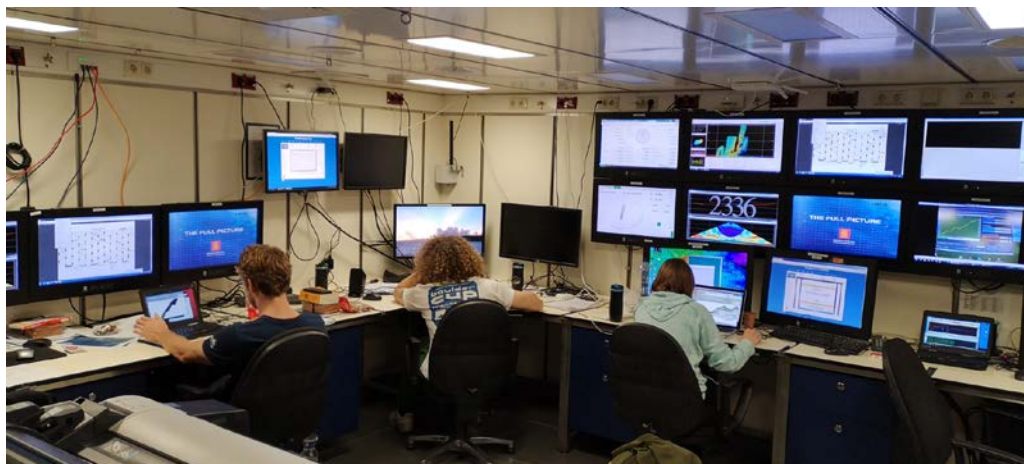
Watchstander Team (from left to right: Linnert Neunz, FU Berlin, Marcel Hanisch and Alexandra Zeh, both FAU Erlangen) at work in the hydroacoustic lab. With great care, love and passion, they remove outlier signals from the data sets. The corrected data will be integrated into the bathymetric map. (Photo: J. Koepke).
