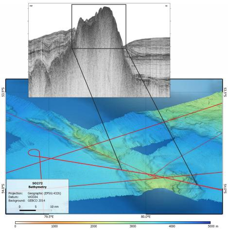
seafloor. This information is necessary to evaluate structures whether images in seismic data are small- or rather large-scale features. The seismic profile shows a hill. The bathymetric data show the spatial structure and extent of the hill, which appears to be related to another hill in the North. Those hills consist of hard rock, most probably of magmatic origin. For us those hills are important because they constitute obstacles for the flow
