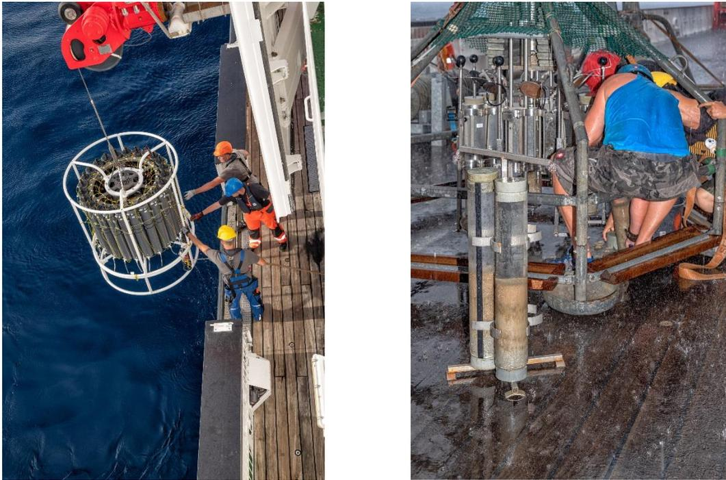
Fig. 2: Water sampling (CTD rosette) and short sediment cores (from multi corer) on SO269 (Photo R. Prien IOW).
