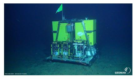
Elevator 1 at the sea floor. The ROV pilots fly to the lander and remove the scientific instruments to deploy them at selected spots on the sea floor. At the end of the measurements the instruments are placed again on the elevator and secured by rubber bands for their lift back to the sea surface.
