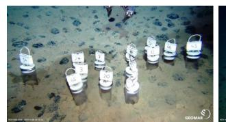
Sediment sampling with push corer.
