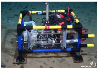
Benthic chamber for the determination of the Microprofiler for the measurement of oxygen oxygen consumption of the sediment.
