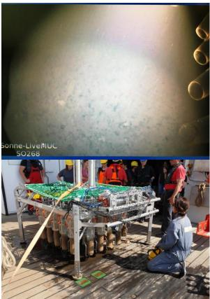
Preparation of the equipment (Elevator-Lander with Launcher, box corer and multicorer) on deck as well as the first video-guided deployment of the new multicorer.
