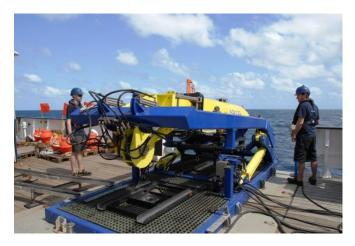
Launch and Recovery System (LARS) for deployment of the AUV ABYSS on the starboard side of RV SONNE.
