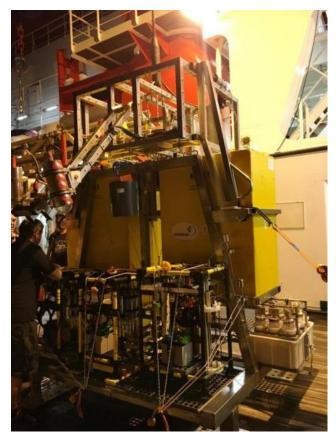
Right: Elevator-Lander with launcher on top.
