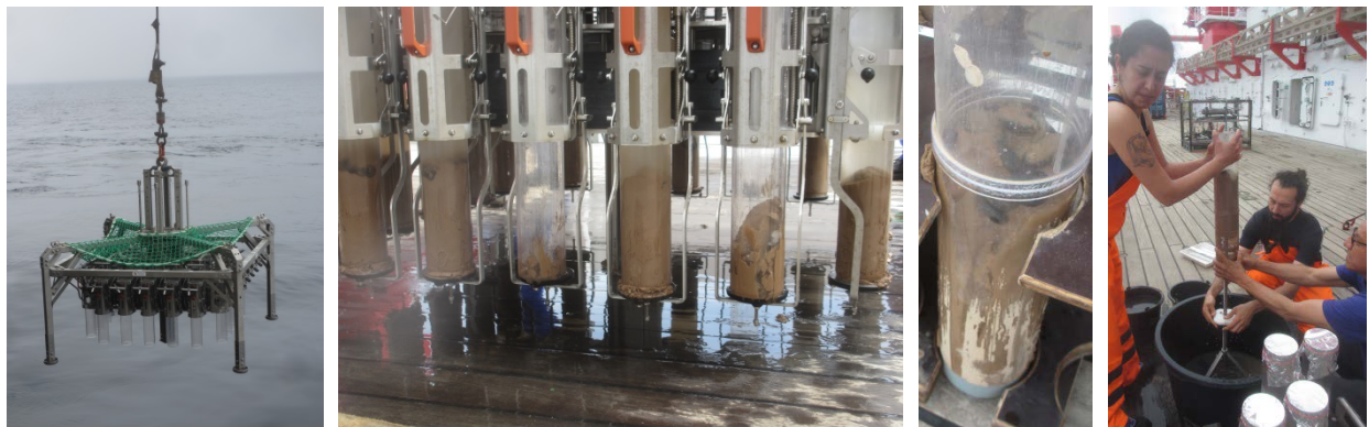
Figure 3. Der Multi-Core Sediment Collector before and after a deployment and the separation of a core's upper 10 cm, which here contains small Mangan-rocks, for future examinations in laboratories
