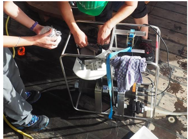
Figure 10 McLane in situ pumps during deployment and sample collection after taking them on board after successful sampling.
