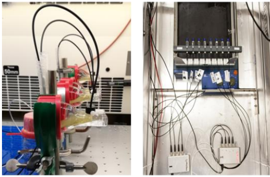
Figure 19 Gas-sealed Oxygen chambers (left) and oxygen profile after incubation of plastic-colonizing biofilms for 10 h in light/dark phases (right).
