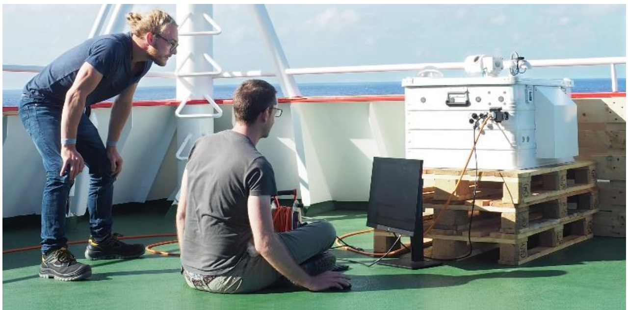
Figure 7 Solar spectrometers operated during SO 268-3: an handheld sunphotometer (upper left), 3 MAX-DOAS type instruments (top center and right) and a fourier-transform spectrometer (bottom)
