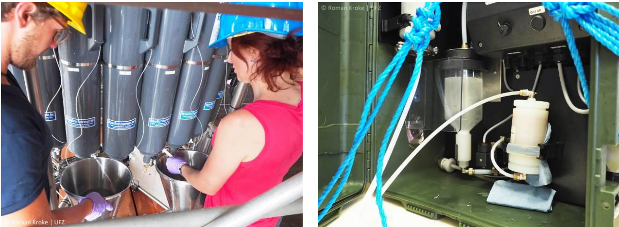
Figure 13 Water was submitted to the LV-SPE either from the ship's seawater supply or from the CTD/Rosette (left) to process deep sea samples. The pollutants from 50-100 L of seawater were enriched on a sorptive phase
