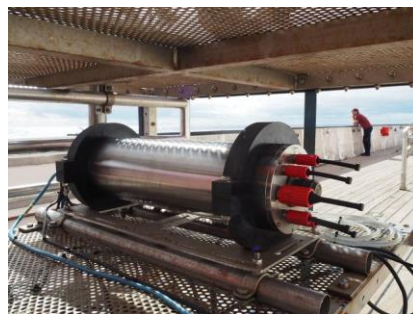
Figure 17 The OFOS system on the working deck (top) and evaluation of the pictures (bottom).
