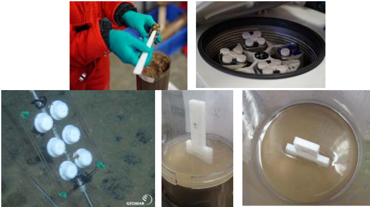
Photos (Sophie Paul, Katja Schmidt, ROV Kiel6000): (top row) Filtration techniques: (left) filter tower, (middle) ultrafiltration, (right) syringe-filtering under the clean bench. (center row) From sediment to clear porewater: (left) sampling in the cold room, (right) centrifugation. (lower row) Passive samplers for the water column at the seafloor (left) and for the porewater in a MUC liner (center and right).
