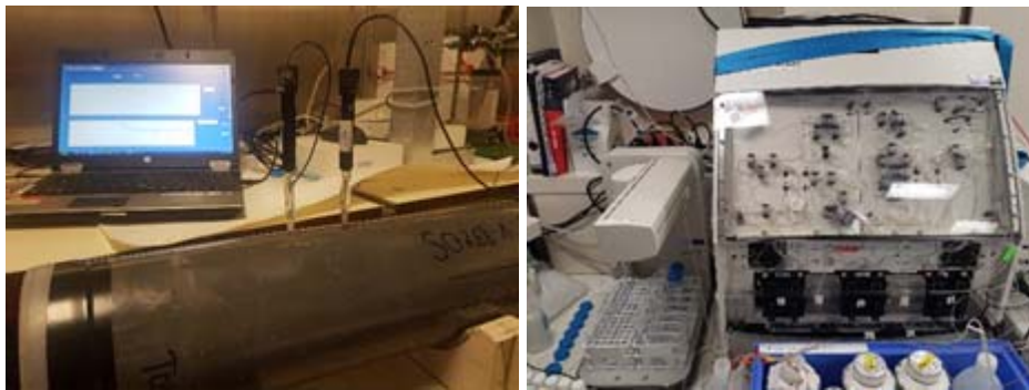
Photos (Jessica Volz): (left) Measurement of oxygen concentrations in long sediment cores using amperometric sensors. (right) Seal Analytical QuAAtro39 segmented flow analyzer used for the determination of nutrients in the pore water.
