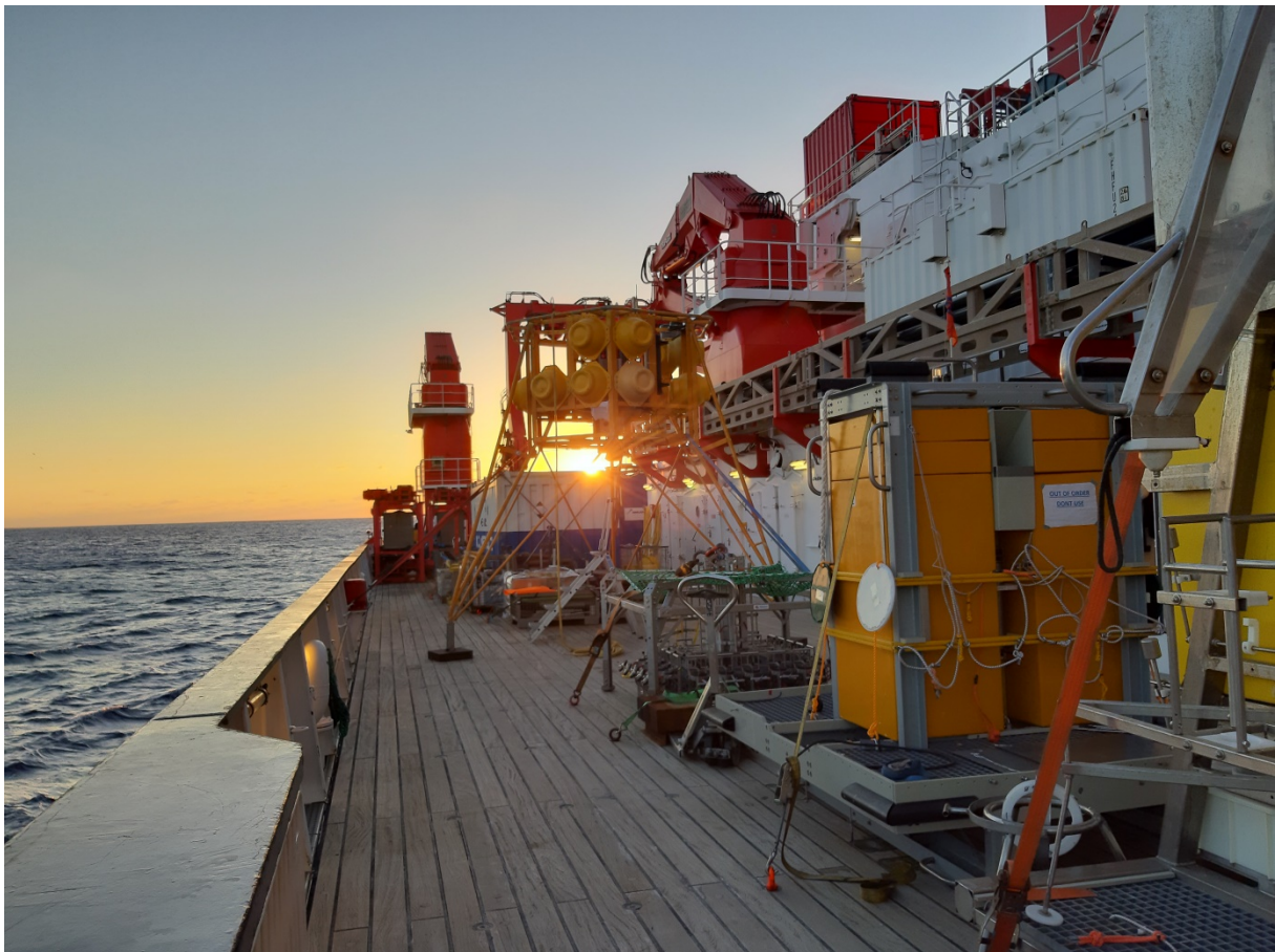
Photo (Steffen Niemann): Benthic lander systems and the multicorer on deck of RV SONNE.
