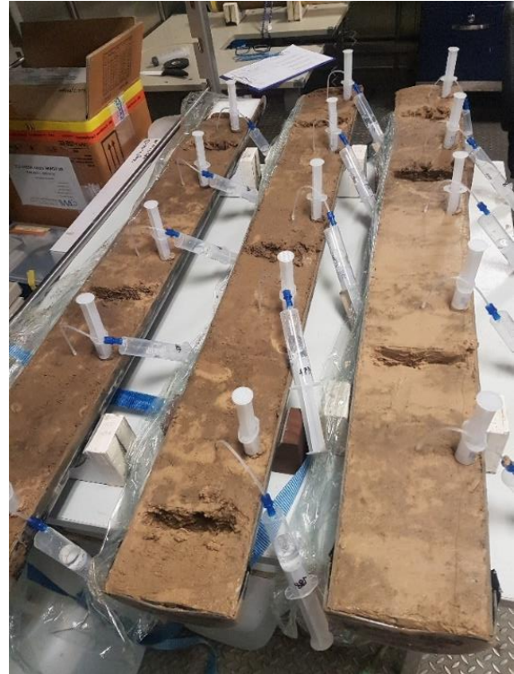
Pore-water extraction with rhizons. Samples for centrifugation have already been taken from these cores – visible where the holes remain in the sediment (right).
