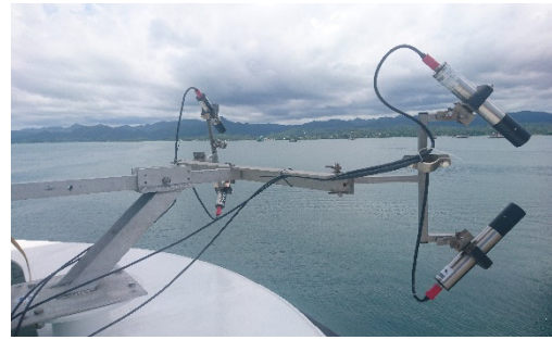
Fig. 1: Radiometer setup onboard RV SONNE (Picture: D. Voss).
