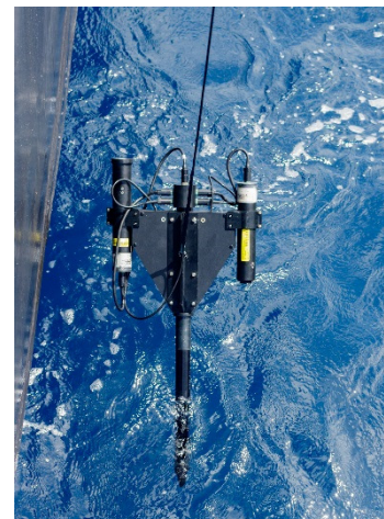
Fig. 2: Satlantic Profiler at the aft the ship. With little speed the instrument will be brought away from the ship (Foto: S. Dörner).
