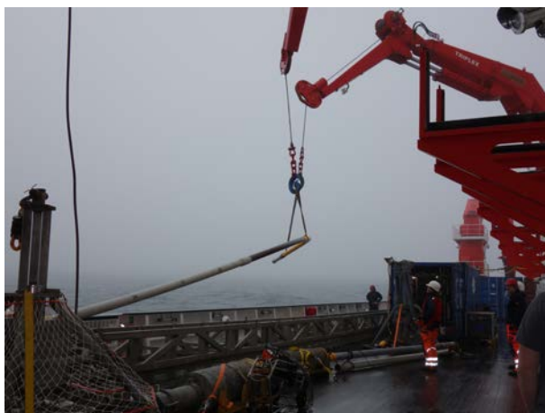
Crane dancing: The retrieval of bent core equipment on deck requires tact.
