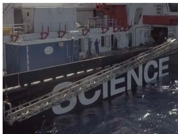
The lowering frame used to deploy sediment corers on RV SONNE.
