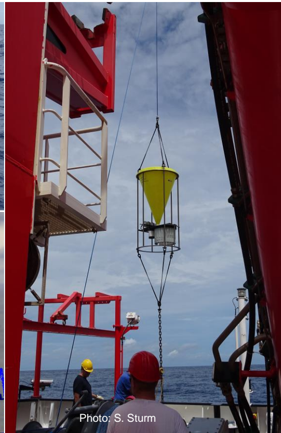
Upper left: floats of the sediment trap mooring after surfacing in the UKSRL license area. Right: hoisting the upper sediment trap onto deck at the aft of RV SONNE. Lower left: graphic representation of the CTD tow-yo profile along the slope of a 2100-meter-high seamount in the German license area.
