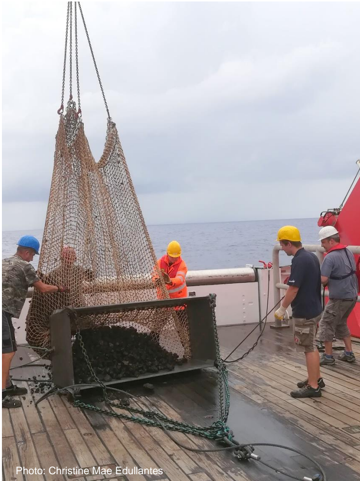
Recovery of the dredge after deployment at a water depth of 4100 meters.
