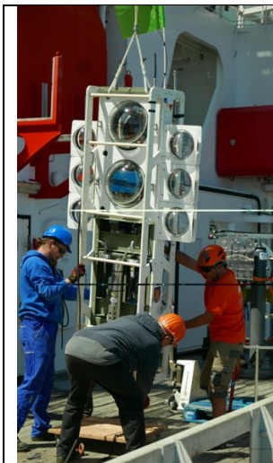
Nano-Lander for collecting water samples at the trench bottom (Foto: M. Schlösser)
