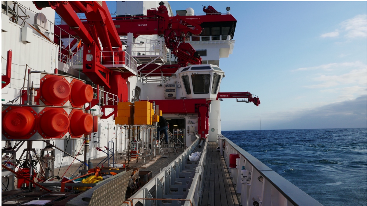
Figure 1: Three different Lander systems for abyssal and hadal in situ measurements are prepared for their first deployment
