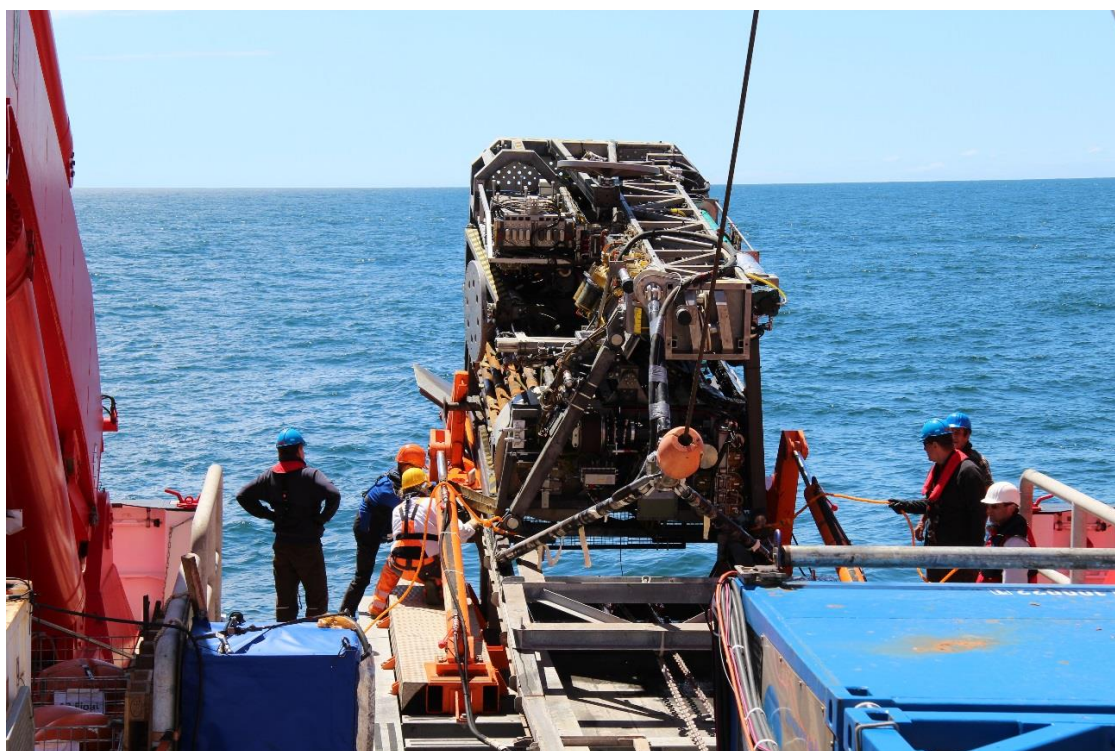
Figure 2: Haul onboard of the seafloor drill rig MARUM MeBo70 on RV SONNE. (Photo: Sabine Kasten)
