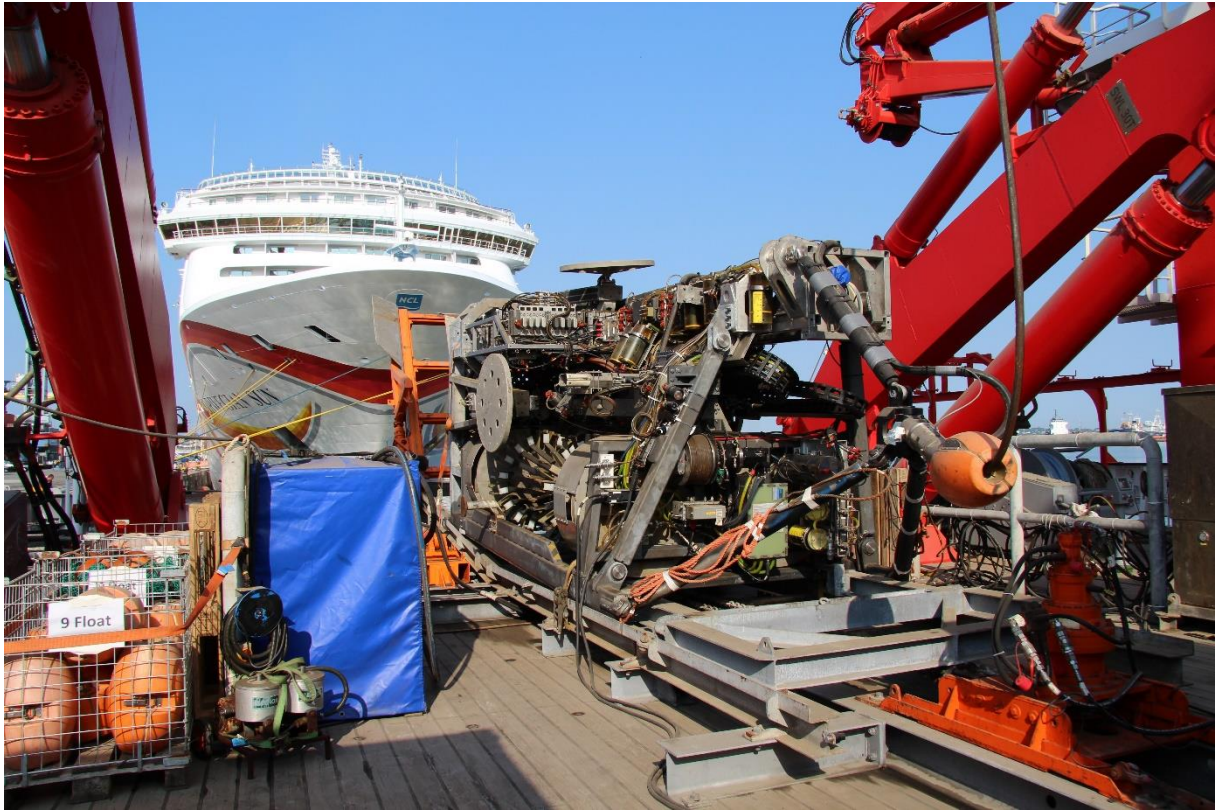
Figure 2: Assembly of the seafloor drill rig MeBo70 on the RV SONNE in Montevideo. In the back is the cruise liner NORWEGIAN SUN (Photo: Sabine Kasten).
