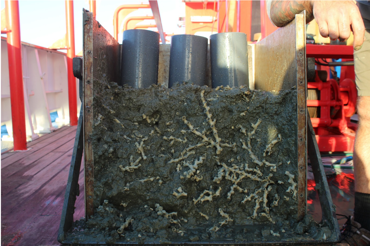
Fig. 2: Side view into an opened giant box corer with plenty of deep sea coral fragments (photo: Janina Bösche).
