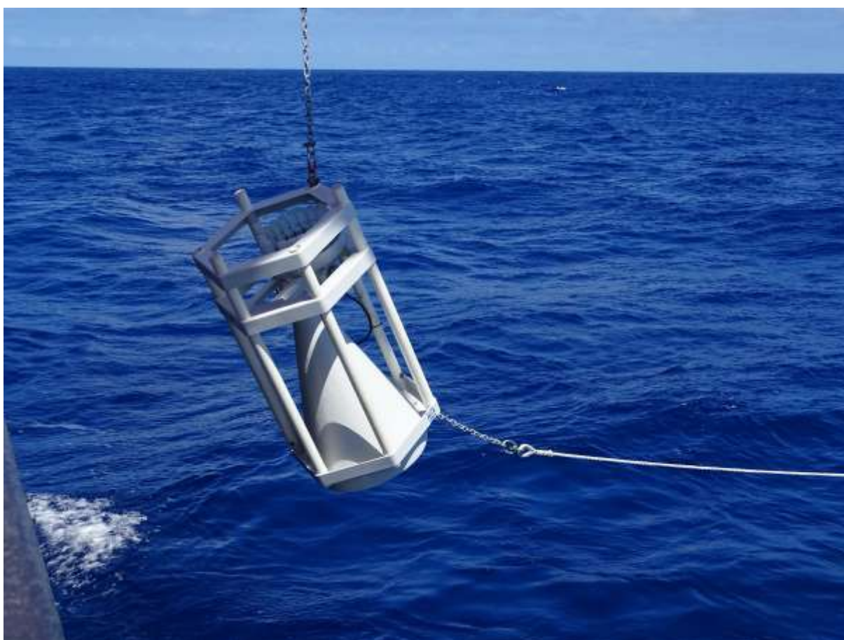
Deployment of a sediment trap for the measurements of particle fluxes close to the seafloor in cluster 1 of the German license area.
