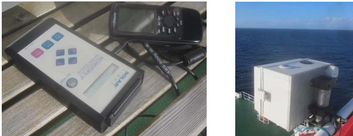
Figure 1. the MICROTOPS sun-photometer with an associated GPS (left) and the cloud-camera box (right) with a normal (visible image) picture sensor and with a thermal (heat sensing) sensor
