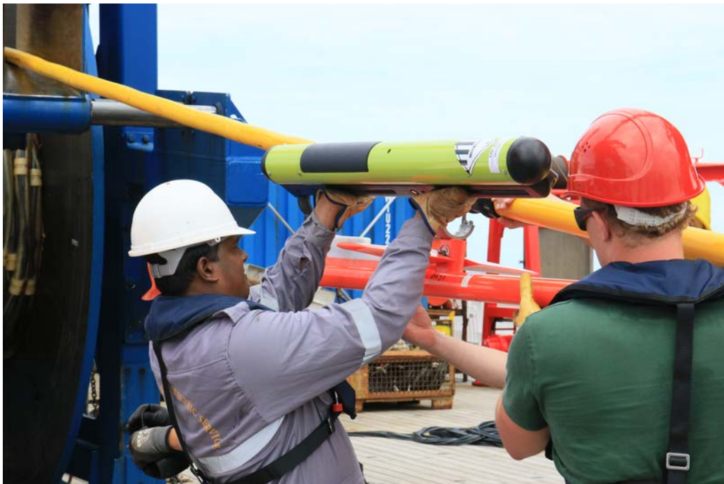
Fixing of a "bird" and a streamer recovery device at the streamer. (Photograph: Masakazu Fujii)
