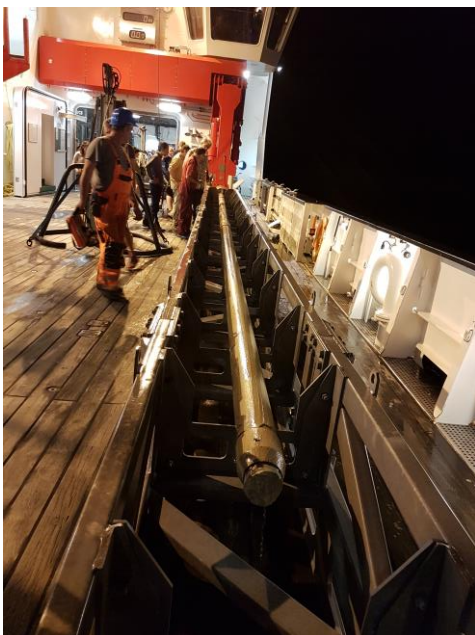
Gravity core GeoB22218-1 being recovered (left) and described/sampled (right) on deck.
