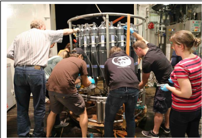
Many work groups sample the Niskins from the CTD deployments for onboard and home lab analyses of plume tracers and other hydrothermally derived components.
