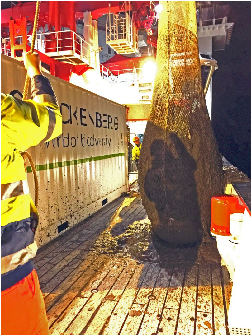
Figure 2: The Agassiz trawl is heaved back on board. After the last, very deep (> 9500 m) station the net is extremely full. These metric tons of mud from the seafloor kept the scientists busy for the rest of the night and half of the day sieving. (c) Angelika Brandt
