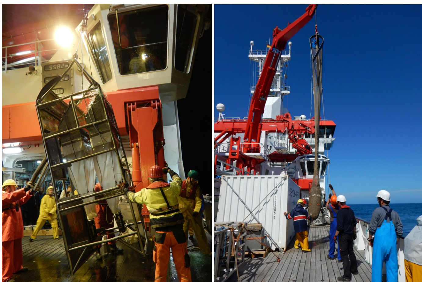
Figure1: The epibenthic sledge (EBS) „META“ (left) and the Agassiz Trawl (AGT, right) are heaved onto the working deck of RV Sonne after the record-breaking deployments. The fine-meshed nets of the EBS and the wider AGT net held sediment and organisms from 9581 m depth. This was the deepest deployment ever conducted with an EBS. (c) Angelika Brandt
