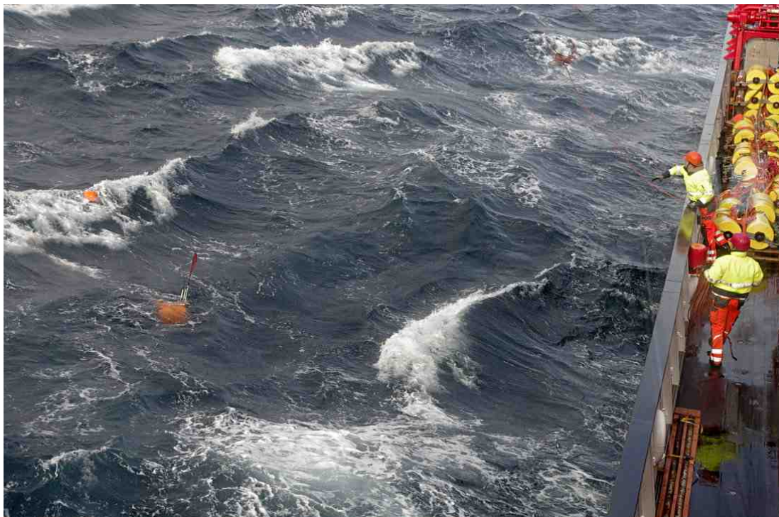
Bringing the OBS's back on board turns out to be quite a challenge for the crew on the bridge and deck. In this case, the enter-hook caught the float-line of the OBS with the first throw by the crew-man (photo: T.N. Gades).
