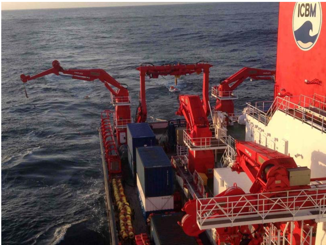
Five types of instruments are being towed by SONNE. From left to right: Passive acoustic monitoring device (PAM), starboard airguns, seismic hydrophone-streamer, portside airguns, magnetometer. Thanks to the wide stern, this tow configuration is possible without the danger of cable tangling.
