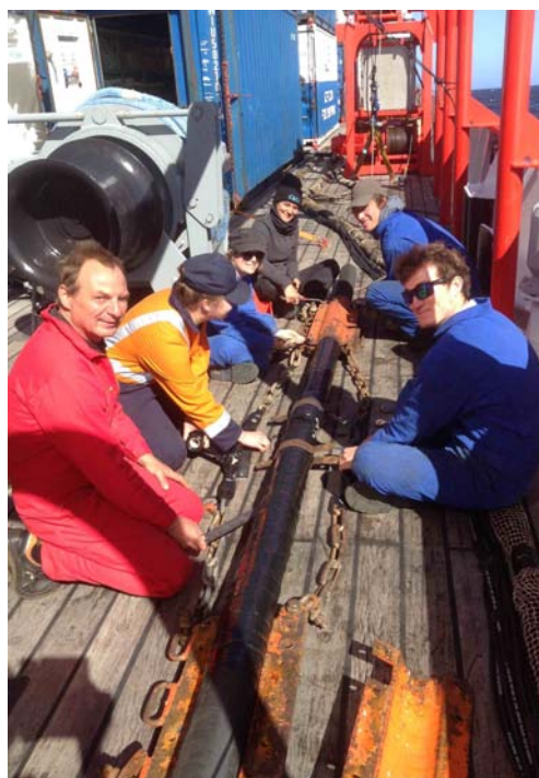
Repair work at one of the airgun umbilicals.
