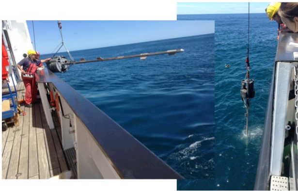
The heat-flow probe with its high-precision temperature sensors is being brought to the seafloor to measure the temperature gradient in the sediments.
