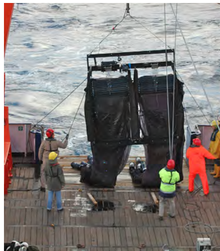
Fig. 2 Deployment of the 1m 2 -double-MOCNESS
