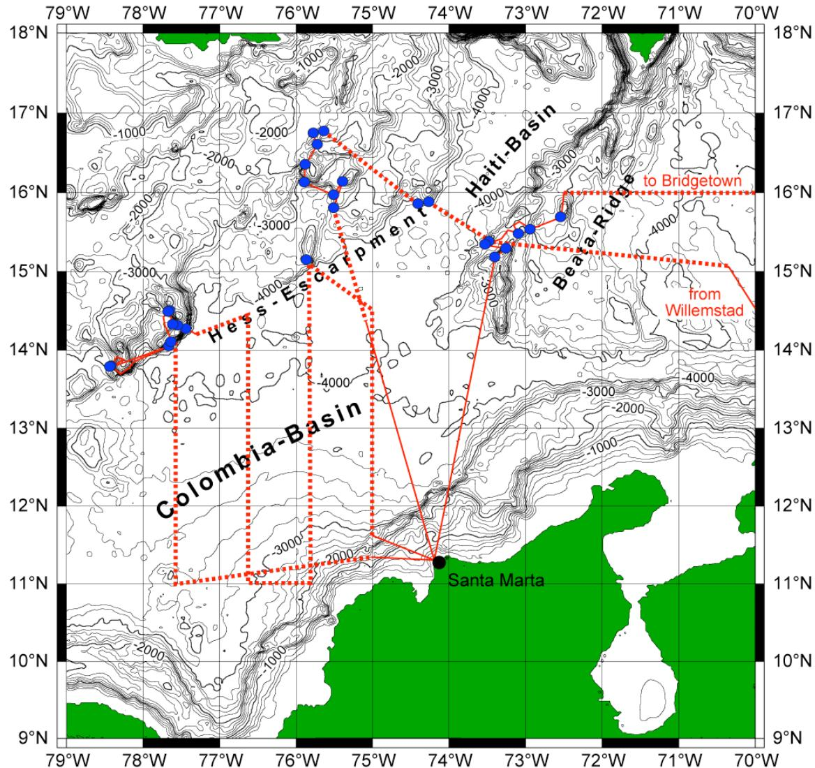
Ship track of RV METEOR cruise M81/2B (thin red line) with locations of dredge stations (blue dots). Simrad EM120 and Parasound surveys were carried out on all ship tracks within the EEZ of the Dominican Republic, Haiti, and Jamaica and on most tracks within the EEZ of Colombia. Magnetic profiles are marked by the dashed red line.
