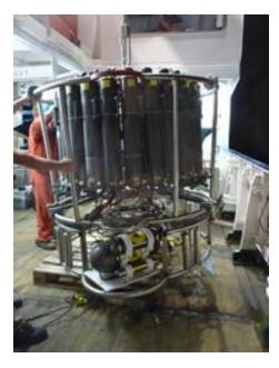
**Fig. 5:** CTD/rosette instrumented with the in situ mass-spec. THETYS.
