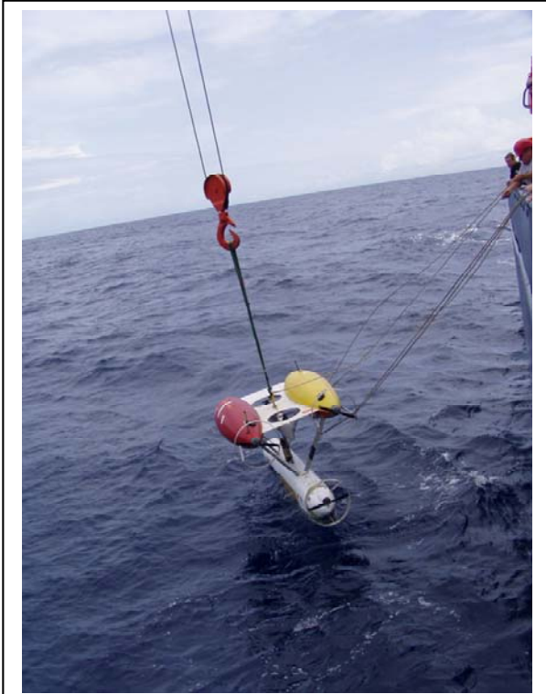
The deployment and recovery of the AUV ABE is practiced.
