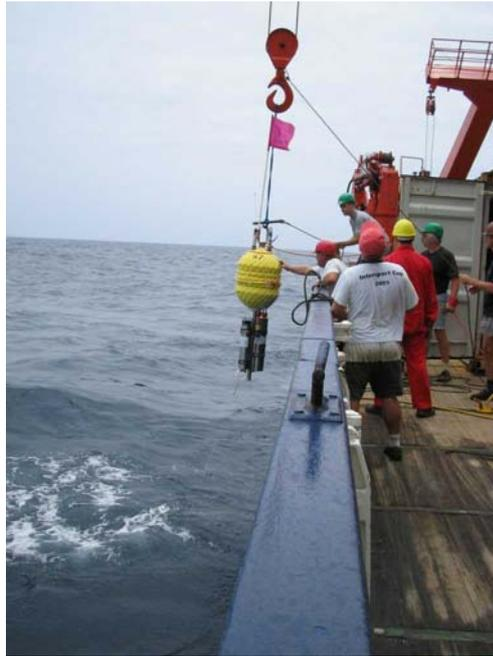
Figure 2: Recovery of an ocean bottom hydrophone.
