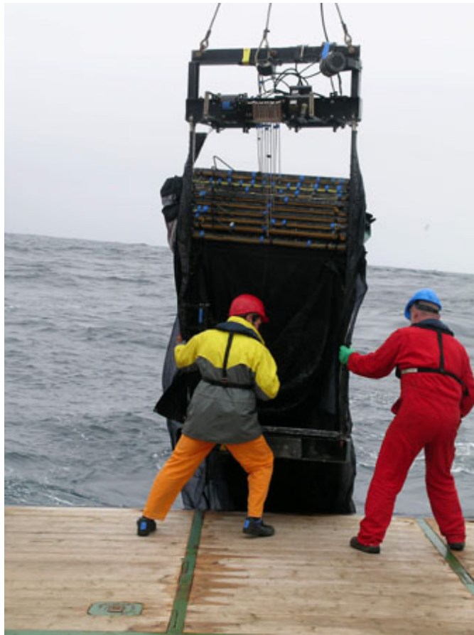
Figure 3: Deployment of the 1m 2 -MOCNESS with 9 netbags.
