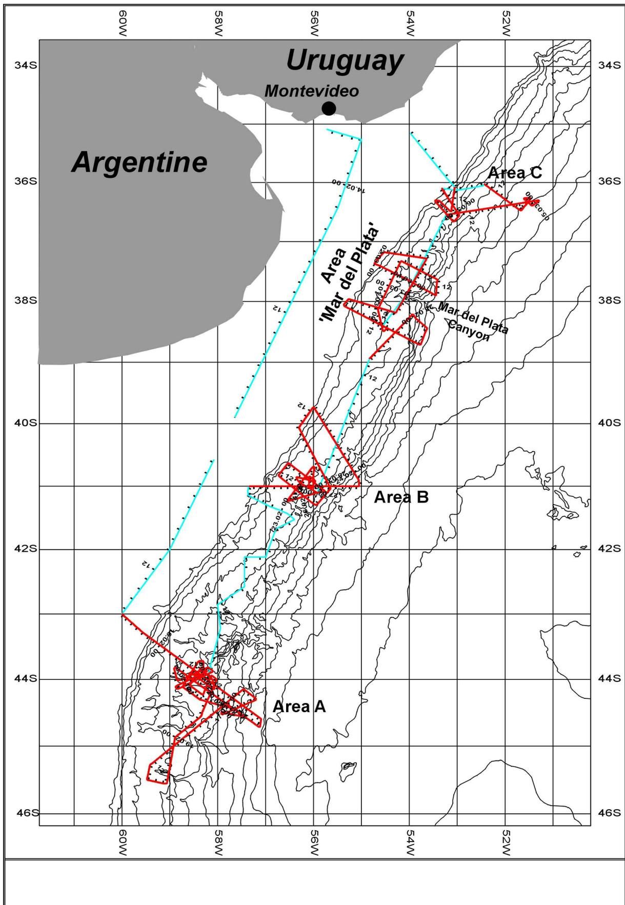
Figure 1: Track Chart of R/V Meteor Cruise M49/2 with seismic lines indicated in red, Hydrosweep/Parasound survey lines in blue. Bathymetry from Gebco Digital Atlas.
