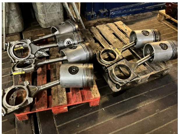
Figure 2: Removed pistons of the diesel generator under repair, of which a total of 4 machines form the heart of the ship (© G. Bohrmann).
