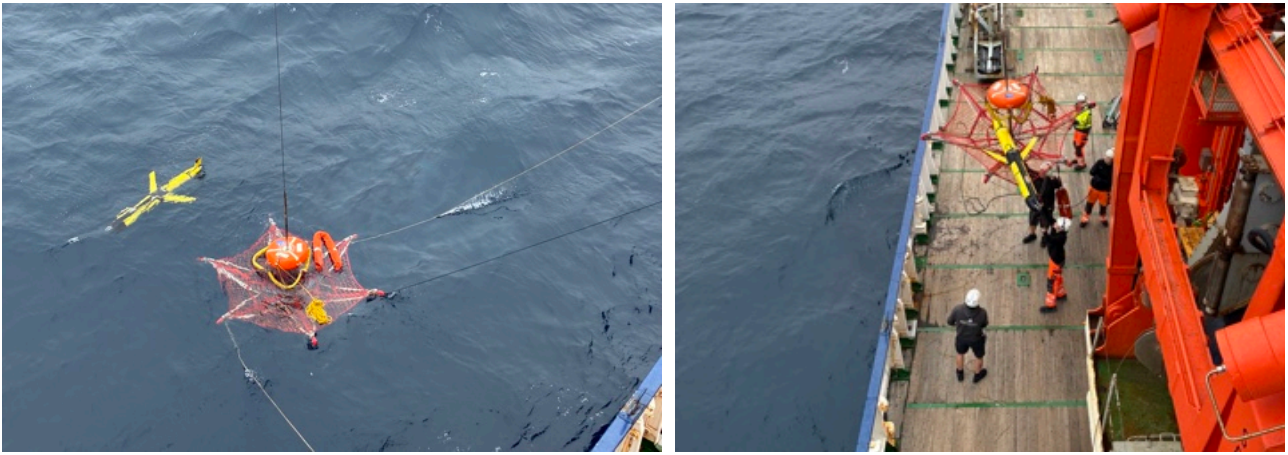
Recovery of the Slocum glider IfM16 on Monday, August 18, using the ship's RLS - Rescue Star, build for recovering persons from the water but similarly useful for equipment.
