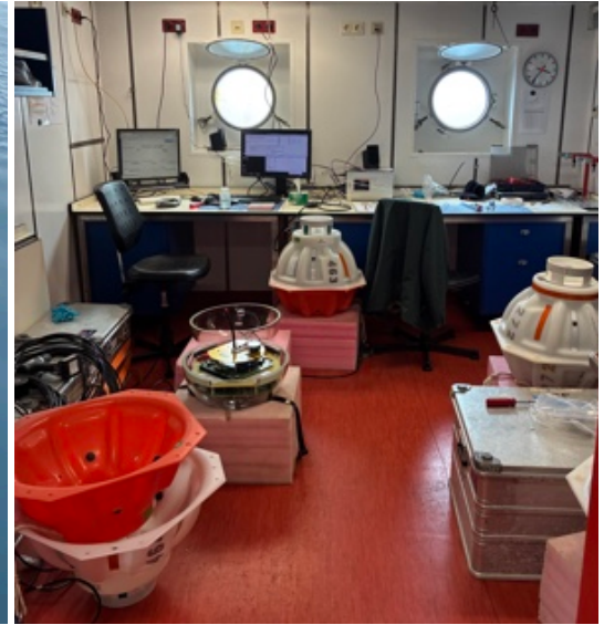
Left: Inverted echo sounder (white) with current meter, mounted below the yellow float alongside METEOR. Right: Inverted echo sounder in the lab for data download.
